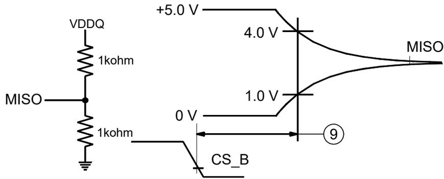
Figure 9. MISO loading for disable time measurement
