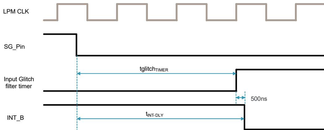
Figure 6. Glitch filter and interrupt delay timers
