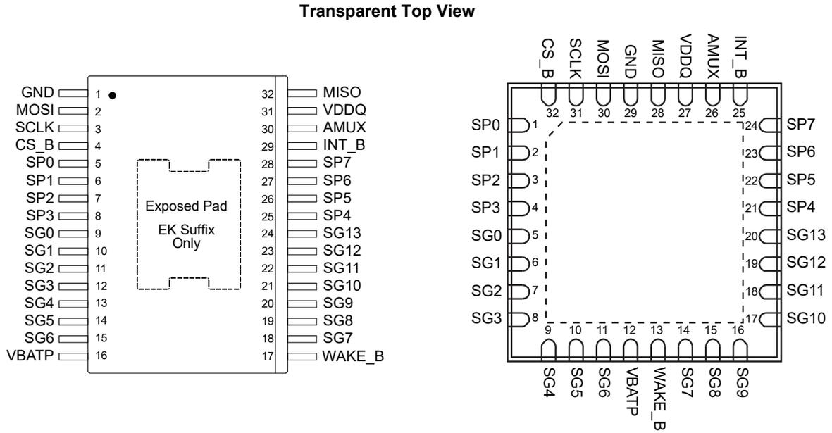
**Figure 3. 33978 SOICW-EP and QFN (WF-Type) pinouts**
