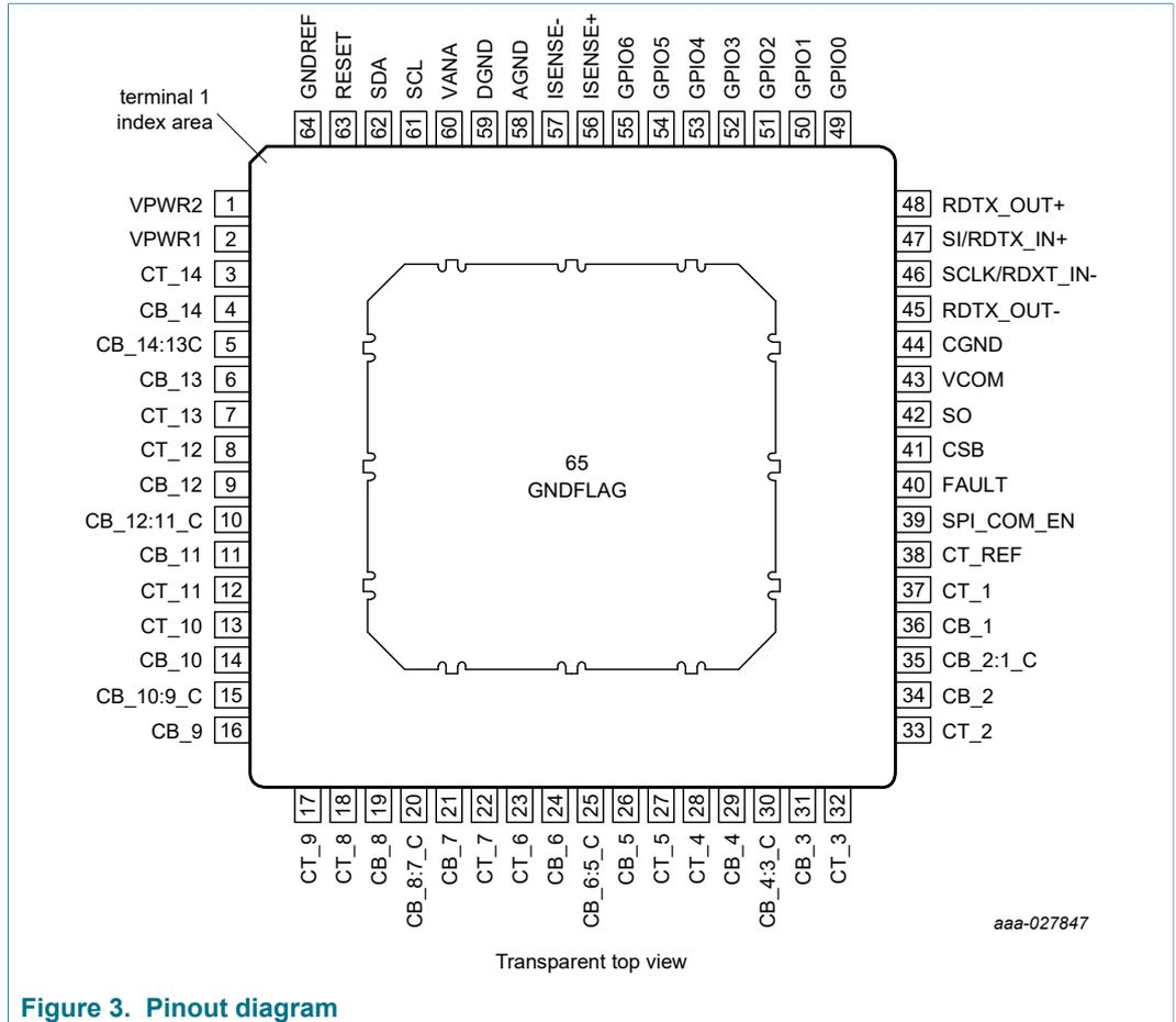
Figure 3. Pinout diagram
